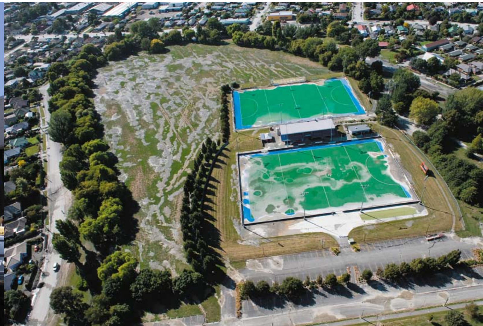
Aerial photo showing extensive liquefaction
